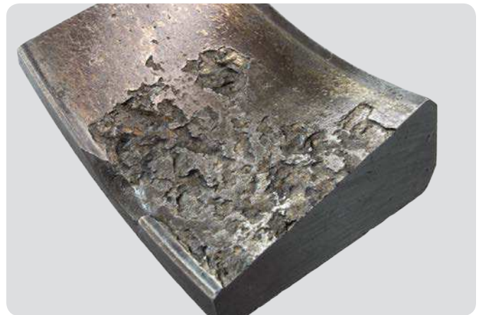
Tapered roller bearing outer ring Inadequate lubricant film leading to surface distress and advanced spalling
