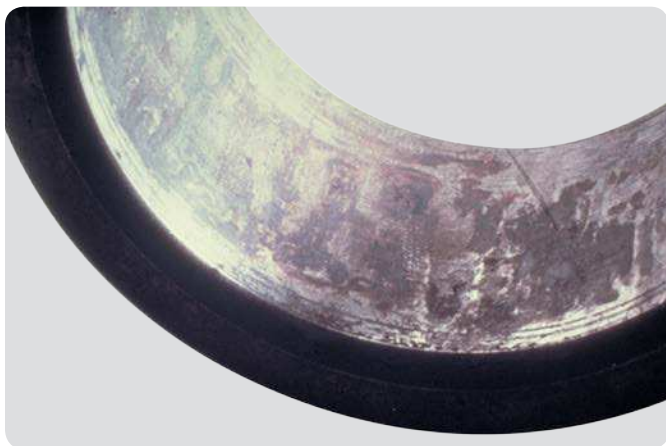
Cylindrical roller bearing inner ring Inappropriate shaft fit (too loose)
