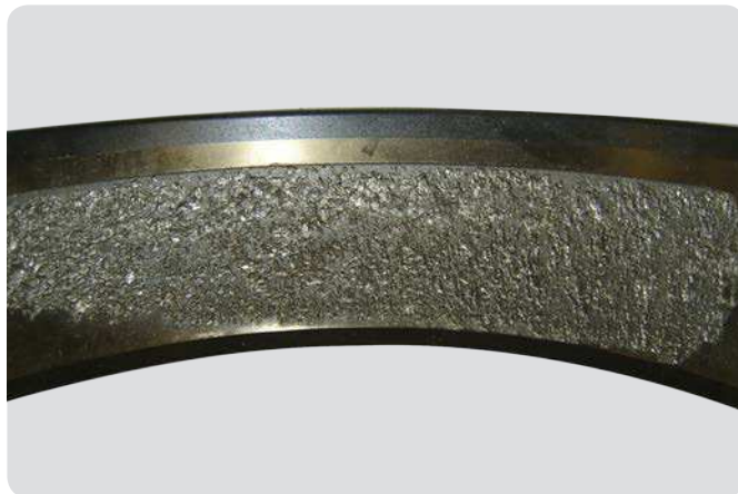
Cylindrical roller bearing outer ring Inadequate lubricant film, some misalignment, advanced surface distress
