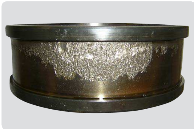
Cylindrical roller bearing inner ring Inadequate lubricant film, excessive misalignment, advanced surface distress
