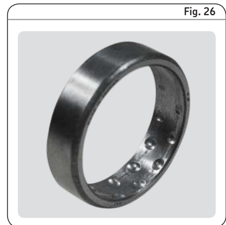
Fig. 26 Severe false brinelling on the outer ring raceway of a self-aligning ball bearing
