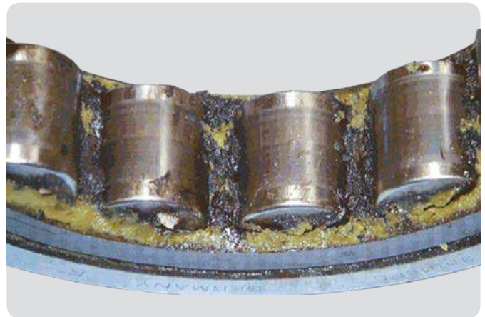
Cylindrical roller bearing outer ring with cage, rollers and grease Current leakage resulted in burnt grease (black) on the cage bars
