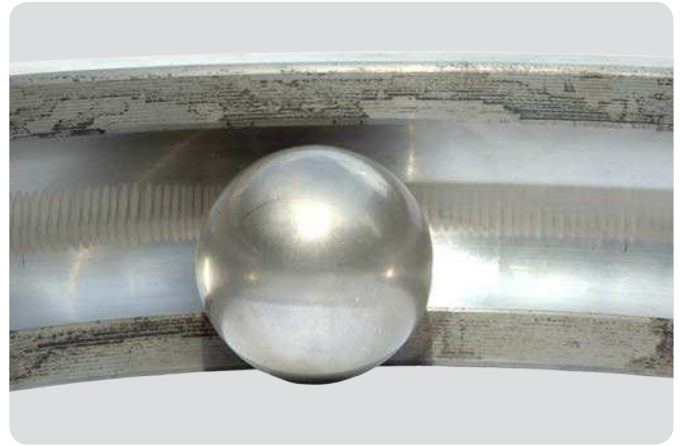
Deep groove ball bearing outer ring and ball Washboarding in the outer ring and dull ball surface
