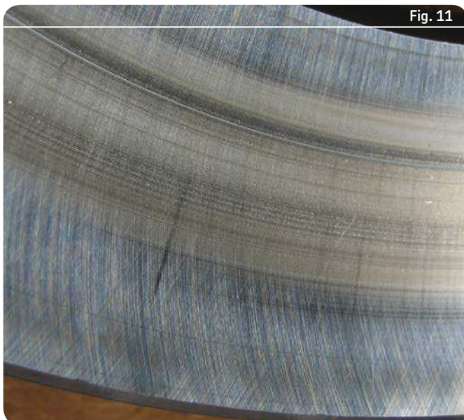
Light abrasive wear on the outer ring of a spherical roller thrust bearing
