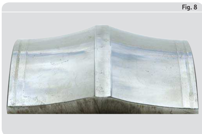
Inner ring: Heavy abrasive wear on the raceways and a circumferential groove at both raceway edges
