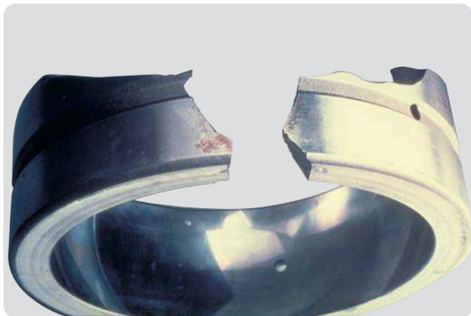
Spherical roller bearing outer ring Fatigue fracture resulting from inadequate housing seat (swarf trapped at the bottom of the housing)
