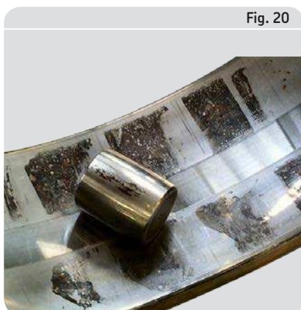
Corrosion on the outer ring and roller of a spherical roller bearing
