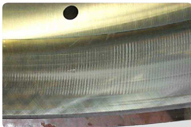
Spherical roller bearing outer ring Current leakage
